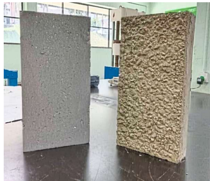
The award-winning palm kernel shell (left) and coconut shell (right) in concrete panels.
