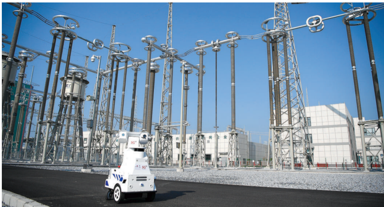
A smart robot, supported by 5G, inspects a power plant in Henan province. LI JIANAN / XINHUA
