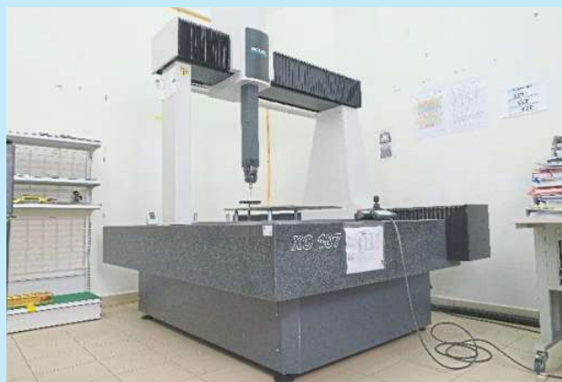
The Wenzel XC 107-CMM is designed for high precision and versatility in measuring components in manufacturing and quality control environments.
